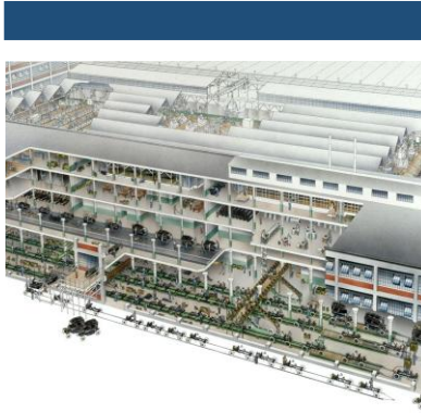
Final Stage of Model T Assembly in Highland Park c.1915. Only in 1913 at Ford's third factory at Highland Park did mass-production begin on a truly large scale. Ford applied assembly line methods throughout the factory to all aspects of car production. (David Kimble's illustration for National Geographic).
